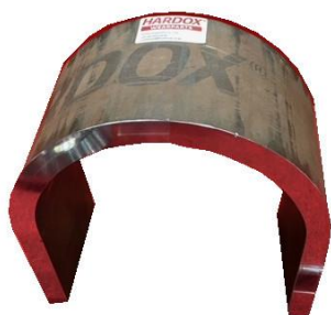
耐摩耗鋼HARDOX50019t-R100曲げ
